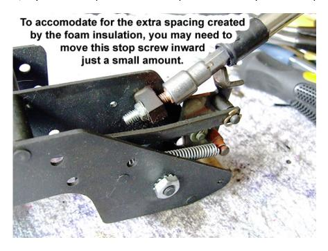
7) After the stop-screw is adjusted inward, you will now need to tighten the nut located on the opposite side of the stop-screw.
