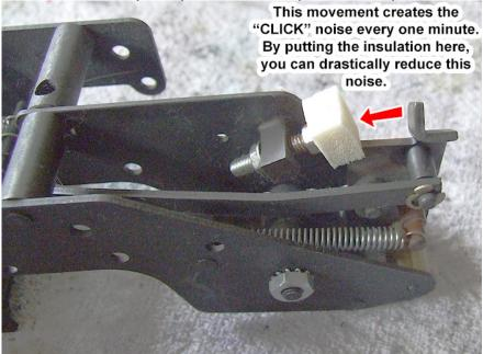
This image shows the cause of the click along with the newly cut foam pad put in place.
