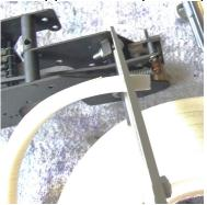
5) Adhere the newly cut piece to the top of the stop-screw as shown below:
